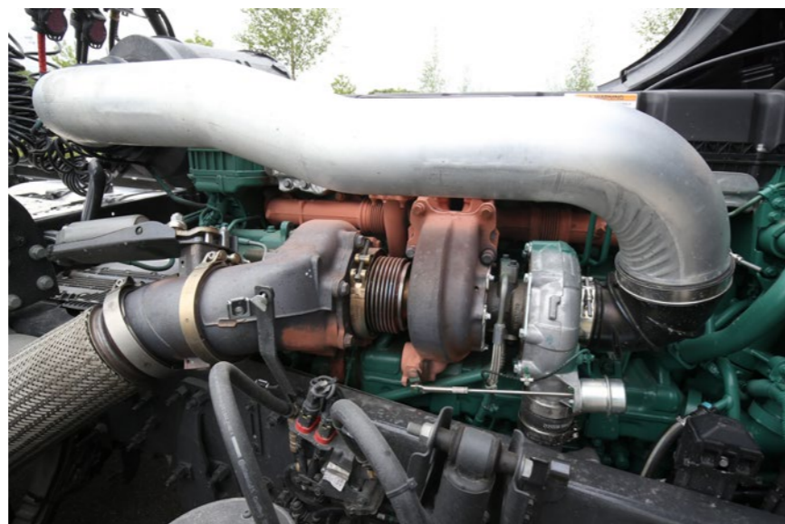
The turbo-compound turbine uses waste heat from the exhaust and provides additional power
